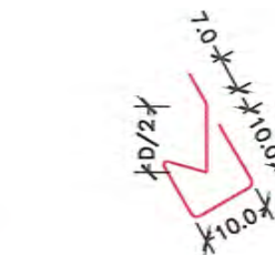
05 CONSTRUCTION JOINT STAND DETAIL SCALE- AS SHOWN
