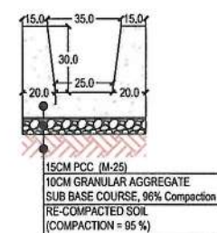
TYPE D PCC DRAIN FOR LINK ROADS
