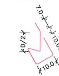
05 CONSTRUCTION JOINT STAND DETAIL SCALE- AS SHOWN
