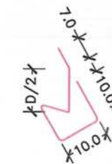
05 CONSTRUCTION JOINT STAND DETAIL SCALE- AS SHOWN
