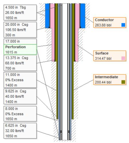
The Contractor shall re-confirm the perforation intervals as per the well logging reports. *Figure 3: Proposed Schematics of Well # 33*
