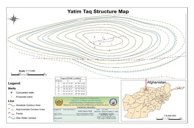
Figure 1: Structural Map of Yatimtaq Gas Field
